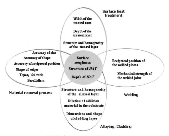
Fig. 2. Objective functions of the material laser processing.
